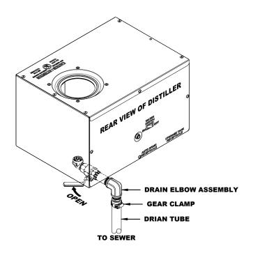
**Manual Drain Valve Location Diagram**
