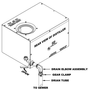
**Manual Drain Valve Location Diagram**
