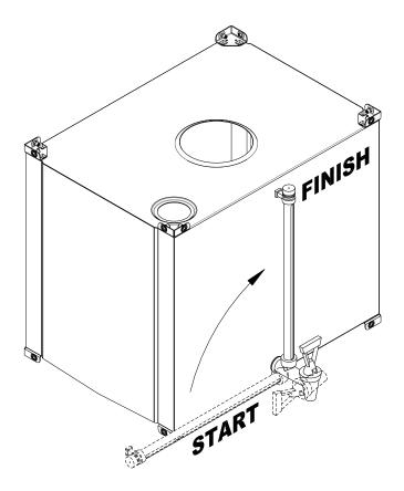
**Tightening Sight Gauge Nut Diagram**
