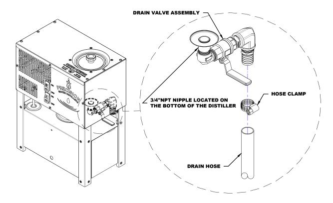
**Drain Tube Removal Diagram**
