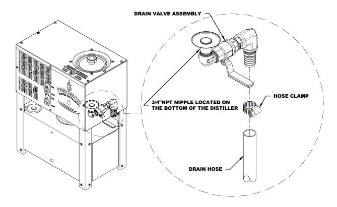
**Manual Drain Valve Tube Installation Diagram**
