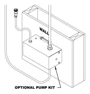
**Pump Wall Mounting Diagram**
