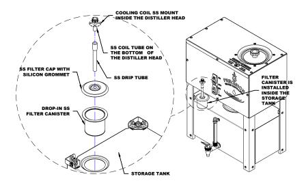
Water Distiller Head Steam Sterilization Diagram
