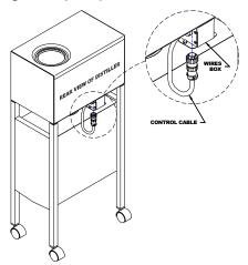
Control Cable Connection Diagram
