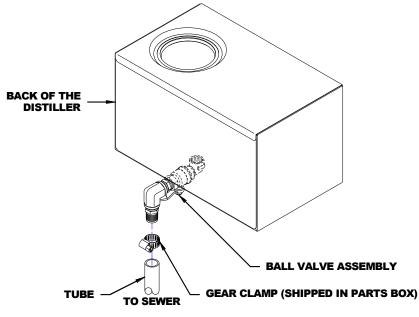
Drain Tube Removal Diagram
