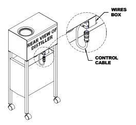
Control Cable Disconnect Diagram
