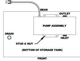
Automatic Pump Mounting Diagram
