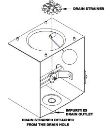
Boiling Tank Strainer Removal Diagram
