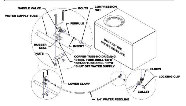
Feed Water Line Installation Diagram
