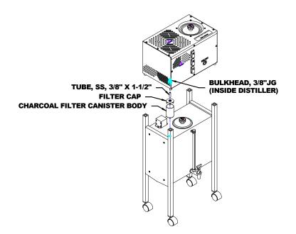
Water Distiller Head Removal Diagram
