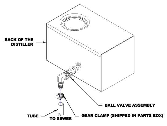
Manual Drain Valve Tube Installation Diagram
