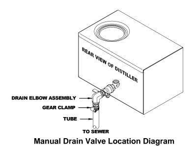
6. Refer to the Manual Drain Valve Location Diagram above. The water distiller boiling tank can be drained by opening the ball valve and draining into a suitable floor drain or container (valve is shown in the close position). The drain may be operated automatically by installation of the Optional Automatic Electric Drain System. See PWS AED-1 Automatic Electric Drain Kit Installation in the Optional Accessories Section for a diagram of the kit and installation instructions
