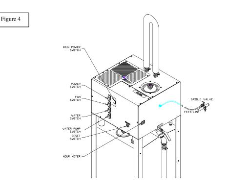
3. Your distiller has been shipped with a sterilization drip tube that is to be placed between the cooling coil and the storage tank. The tube end should be inserted into the storage tank properly. As your distiller continues to heat up, you can sterilize your distiller by simply turning the fan switch off for approximately ½ to 1 hour. Leaving the storage tank lid on. After this cycle is completed, turn the fan switch on and drain any excess water from the storage tank.
